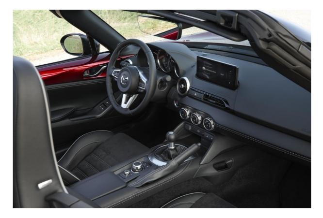
The driver's instrument panel behind the steering wheel has been refreshed with a newly shaped pointer, and a font made clearer and easier to read by the adoption of a higher-pigmentation black Japanese lacquer.
